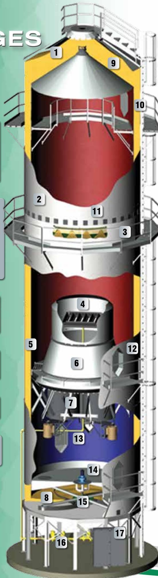
**1** **ROTARY SENSOR** for choke fill or demand fill are standard.
