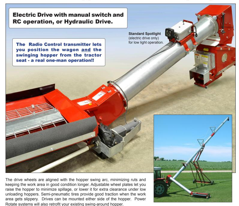
Power Hopper Rotate systems are available for 10" augers with single and twin screw hoppers, and 12" augers with twin screw hoppers. Power Rotate systems will also retrofit your existing swing-around hopper.
