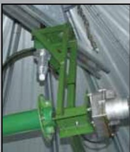
**New pivoting hanger with offset (patent pending) provides more stirring in the center of the bin where it's toughest to dry.**
