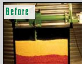
The picture at left shows overdried grain colored red at the bottom with wetter grain at the top. Constant pitch augers pull dried grain from the bottom, mixing it with wetter grain at the top while loosening the grain to increase airflow.
