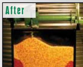
Sukup augers are continuously working forward while moving in and out on the crosstube to ensure all grain is being stirred. During the stirring process a mechanical reversing drive and downward pull of the augers ensure a positive changing pattern.
