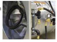
Stainless Steel Flame Sensor is more reliable and lasts longer than flame probes.
